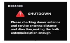
if not working and Self-oscillation get seriously, which overcome ISO and ALC function address range (ALC≥42dB, ISO≥ 42dB), the Sub-band (with Self-oscillation) would be auto-shutdown ass above message, which shows shutdown status (red) for this Sub-band in Menu Page, to protect Base Station wouldn't get interference.
