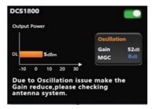
Repeater system will strictly check Self-oscillation degree for all of sub-band and firstly will show abnormal status (Orange) in Menu page, ISO and ALC function would auto generate and if user enter into the soft Self-oscillation sub-band, user could check more details about Self-oscillation with recommend info.
